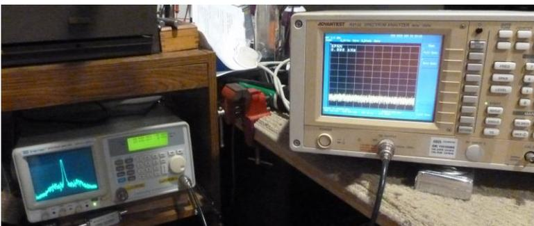
I tested the 3132 by connecting to the tracking generator of my Instek at 30, 300, 600, 900 and 1000 MHz and tuning the 3132 to each frequency. In each case the signal was exactly where it should be on the 3132.
